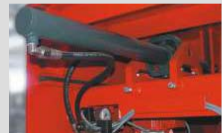
Integrated Hydraulic System with cylinders mounted on universal joints
