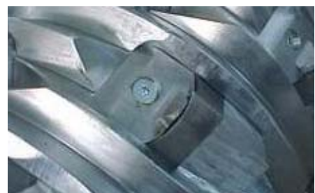
V-Rotor with mounted/bolted knifeholders for abrasive materials
