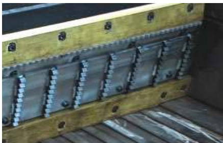
Pronged rail in the ram to avoid material spinning
