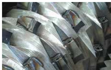
V-Rotor with welded knifeholders for universal use
