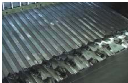
Serrated Ram for thin material
