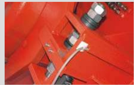
Gearbox Limit Switch works in conjunction with the Reverse Counter as tramp metal protection
