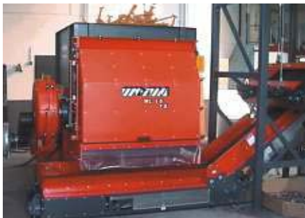
WLK 15 Shredder and conveyor belt with magnetic shut-off switch
